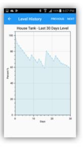
The mobile app can be used in list view or tank view. Level history graphs can be seen for each tank. Pumps can be controlled by tapping the list entry for the pump you want to control.
